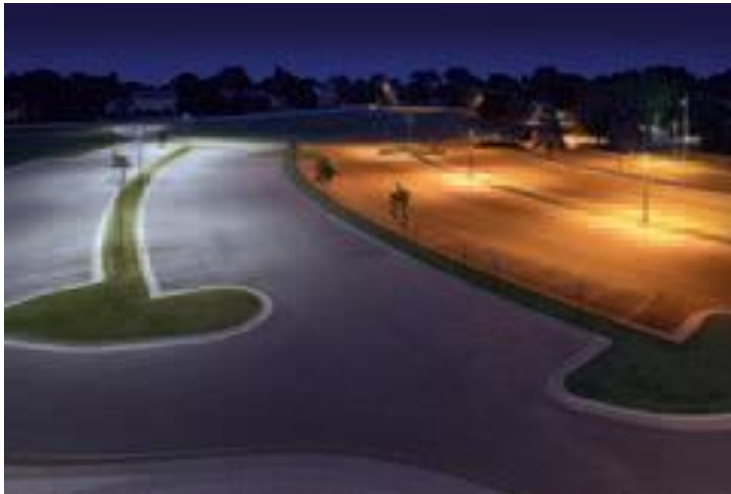
LED (left) vs HPS (right) Source: Beta Lighting & EERE
